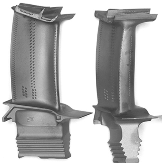
Fig. 9 Rolls-Royce Trent 800 HPT blade after 8299 h (cleaned) (reproduced by permission of Rolls-Royce, plc.).
